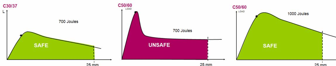
Figure 5: Examples for energy absorption results with FRC with low and high compressive strength
