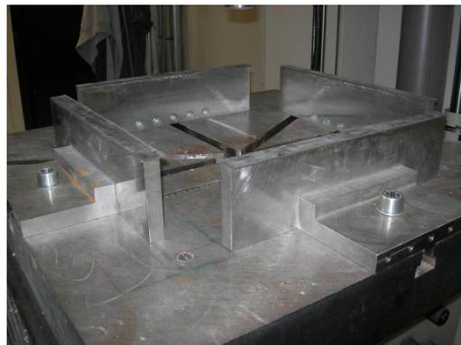
*Figure 2: Support for EN14488-5 test*
