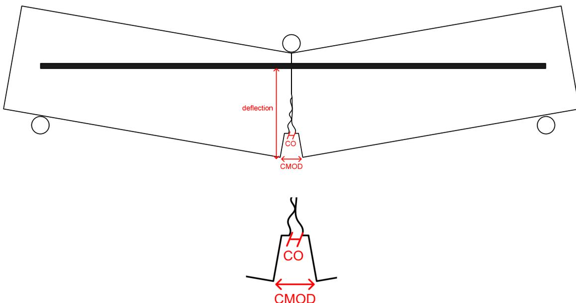
Figure 8: Definition of crack opening, CMOD and deflection
