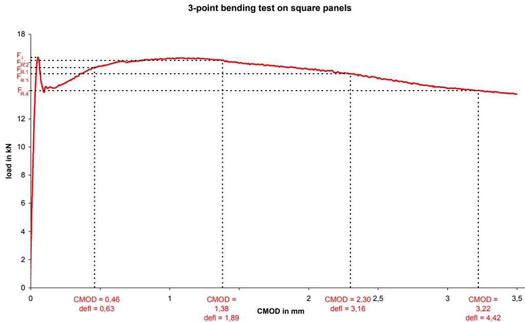
Figure 7 - Load-displacement curve of a 3-point bending test on square panels
