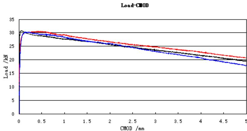
Figure 11: Three curves for PANEL with 40 kg/m<sup>3</sup> SF [7]
