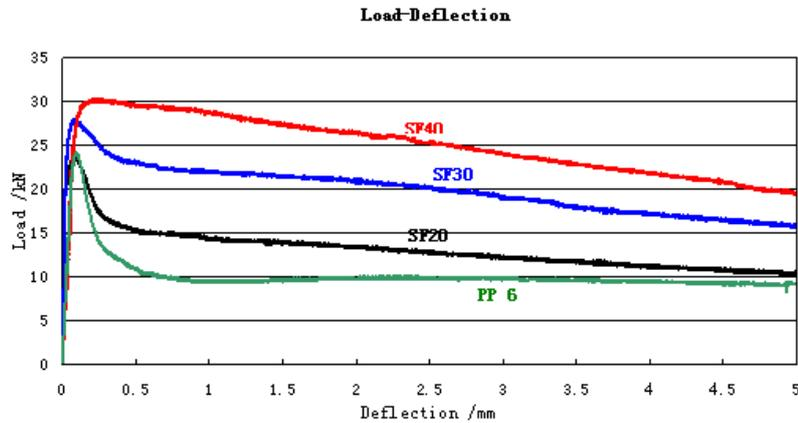
Figure 9: Comparison of Load-Deflection curves of FRC panels with different fibres. Each plot represents the mean result for each set of nine panels.[7]
